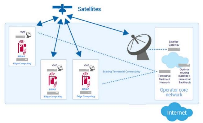
Figure 14: Backhauling and Tower Feed
