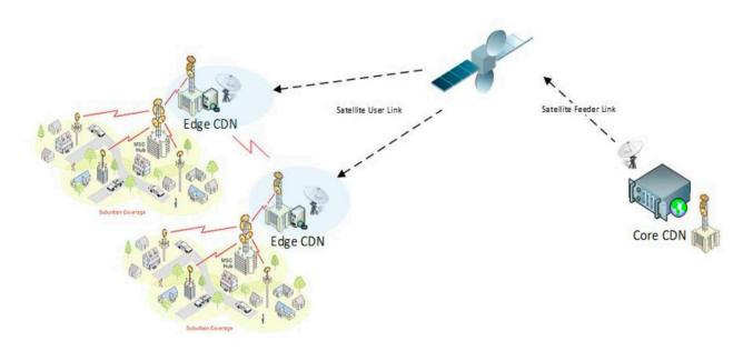
Figure 15: CDN Operation via Satellite Only
