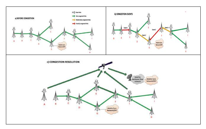
Figure 11: Deployment scenario demonstrating how satellite solution can resolve congestion problem<sup>4</sup>
