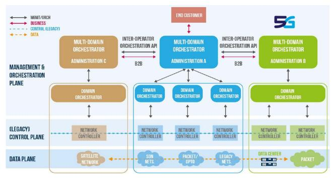
Figure 17: Satellite Service Delivery orchestrated as part of a multi-network (source: 5GIA [5])
