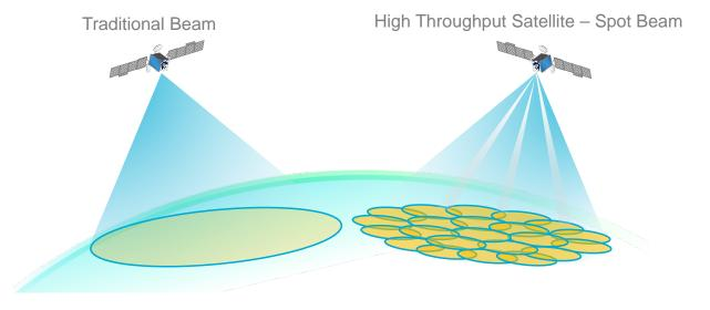
Figure 16: Difference between Traditional Satellite Beam and HTS Spot Beams
