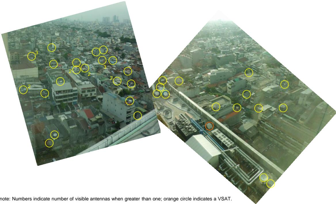
note: Numbers indicate number of visible antennas when greater than one; orange circle indicates a VSAT.
