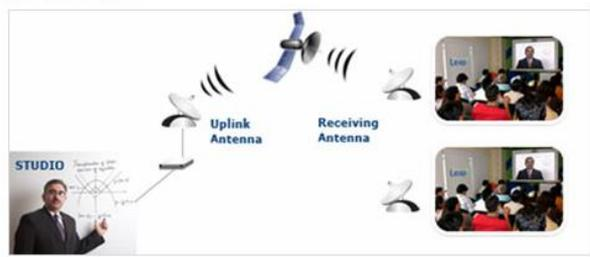
The diagram illustrates the Leap VSAT system. It shows a 'STUDIO' where a teacher is presenting. An 'Uplink Antenna' is connected to the studio, and a 'Receiving Antenna' is connected to a classroom where students are learning. The diagram also shows a satellite in orbit between the antennas.
